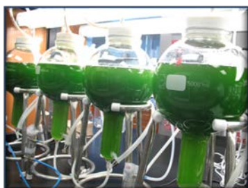
Fig. 1. Biomass production of Stichococcus bacillaris strain siva2011 in 5L bioreactors (working volume 4L each)
